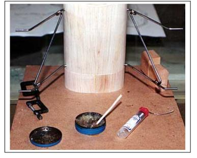
the assembly about to be soldered. The completed assembly has cooled and plastic clamps have replaced the metal ones.
