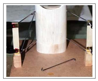
cabanes are supposed to be perpendicular to the thrust line (side view). The brass and plywood pieces are clamped in place temporarily to ensure the cabanes are properly spaced. When I was satisfied with the alignment I wrapped and soldered the diagonal strut to both the front and rear cabanes. I used rosin-core electronics solder.
