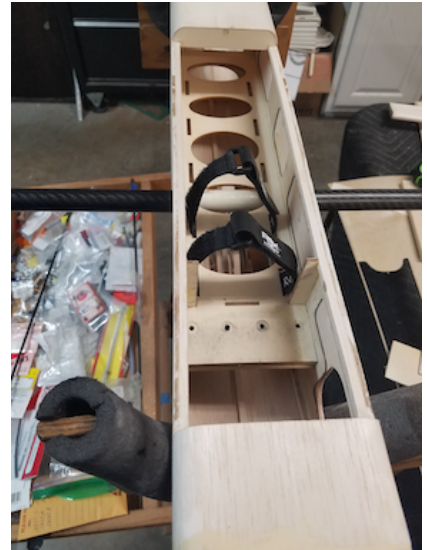
From upper left: Dirty Birdy motor installation; Dirty Birdy battery installation; Battery tray on a model under construction; Warlock 40 (another Bride design) motor and battery installation.
