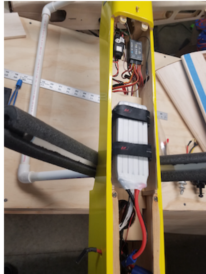
From upper left: Dirty Birdy motor installation; Dirty Birdy battery installation; Battery tray on a model under construction; Warlock 40 (another Bride design) motor and battery installation.
