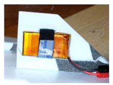
The battery is mounted using hook and loop tape (Velcro). Cut slits in the nose fin to slip the velcro though the slits. In addition to this, I stuck the a piece of the hook side to the fin and another piece to the battery for added holding power.
