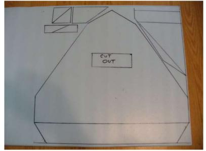
You'll need a sheet of 1/4" blue foam, marker, ruler, Xacto or similar knife, soldering iron and solder, hot-melt glue gun and glue, and fiberglass packing tape. The schematics included are really just guidelines, they're for the Warp that I'm currently flying. You can round corners, change angles, and change any dimension you like, but keep in mind that any changes you make, you'll be changing how the plane flies.
