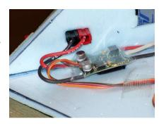
The servos are mounted by first surrounding the servo with heat-shrink tubing and then hot melt glue. The heat-shrink tubing makes it much easier to remove the servos if needed. Just cut the tubing and the servo comes free. (Editor's note: Neat Trick!!!!) The control horns are hot glued onto the rudder and elevator.
