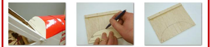
Make sure that your pattern fits, and trim any additional material if necessary. Once you're satisfied with the fit, trace the outline on to a piece of Balsa. The nice part here is that almost all modelers have some balsa on hand, regardless whether you build from scratch, kits, or even ARFs.
