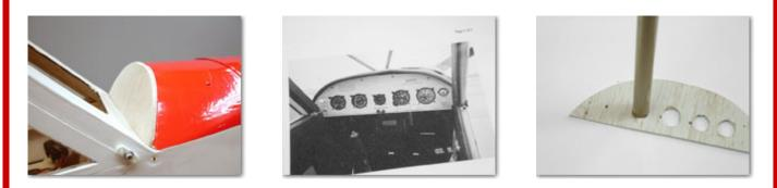
Double check the fit of your new panel at this point. One thing I did on my panel was to sand the top edge flush with the curve of the decking on the nose of me Super Cub.
