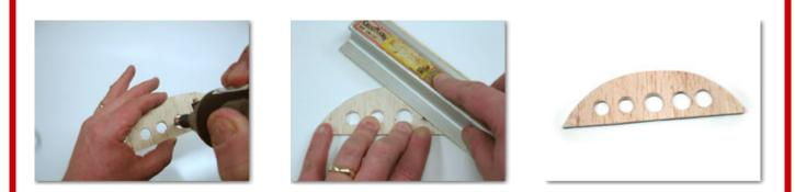
Next up was to finish trimming the holes to the correct size. This is easily done using a rotary tool and a sanding drum or grinding bit. I used two different bits and beveled the edge of each hole to give it a mare finished look. Sand the panel flat now, and get it ready for painting.
