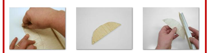
Cut out your panel from the piece of balsa, and sand it to fit. It's nice to have some basic building tools at this point, but a block and a piece of sandpaper will work fine too.
