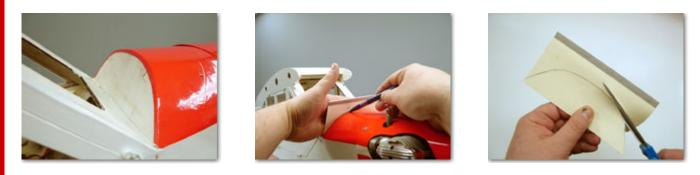
If you're adding your panel to a new airplane before you finish assembly, install it before the windshield/ canopy. If you're adding the panel to a finished airplane, remove the windshield/ canopy. Trace the outline of the panel on to a thick piece of cardstock- I just happened to have an empty check book cover handy, so I used it to trace on. After you have your pattern, simply cut out the pattern.
