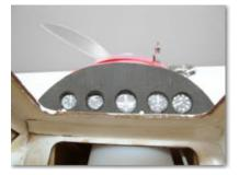
Here's the mostly finished panel. The gauges are glued to the back of the panel with CA. I chose to cut a strip out of a small plastic bag and glued that strip to the panel before the gauges. This gives the gauges a shiny look. After the panel was installed, I drilled two holes and glued in small nails. these simulate the knobs and switches on a real instrument panel.
