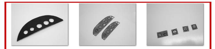
Depending on the panel you're making, and the plane it's part of, you can paint your panel any color you want. I chose to paint mine with a flat black acrylic crafting paint. If your panel is in an open cockpit, you will want to use a fuel-proof paint if the plane is powered by a glow engine.
