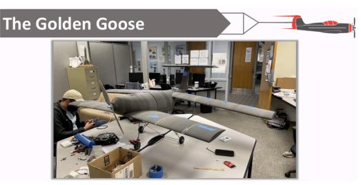
operations test, with mostly good results. All control surfaces worked, and the nose of the plane withstood the torque of the propeller. The center of gravity was slightly off.
