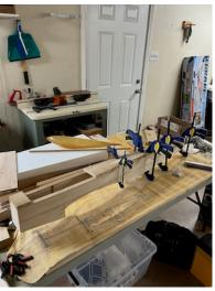
The photo sequence on the previous page shows the fuselage jig, the fuselage sides lined up on the jig along the correct centerline, the fuselage after being removed from the jig, the top blocks being installed (the open space is for the battery access hatch), and the final shot shows the rudder and vertical stabilizer aligned where they will go once the tail surfaces are installed.
