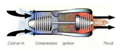
A model jet engine needs to be started with compressed air to initially power-up the turbine. This is commonly supplied from a diver's oxygen tank or something similar. Only when the compressor has reached the necessary revolutions per minute (RPM), can the fuel be introduced into the chamber and the engine can then operate normally.
