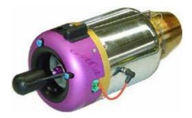
Model rc jets have traditionally lacked the authenticity of having a true jet engine until recent years; previously jets needed to be powered by either gas or electric motors with a propeller (thus spoiling the look of the aircraft), noisy ducted fan or 'pulse jets' (which are more rocket motors than anything else), but now they can be powered by a fully functional jet turbine.
